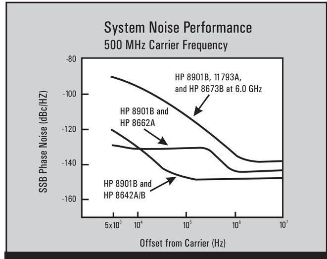
To extend the measurement range to 26.5 GHz, add the HP 11793A Microwave Converter and a low noise microwave source, such as the HP 8673B Synthesized Signal Generator. With this system you can test high-performance sources from 10 MHz to 26.5 GHz.
