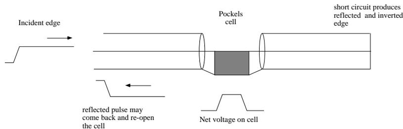
This is like the edge colliding system but the turn off edge is just the turn on edge reflected from a short circuit. The nearest proximity of the short circuit sets the shortest gate obtainable.
