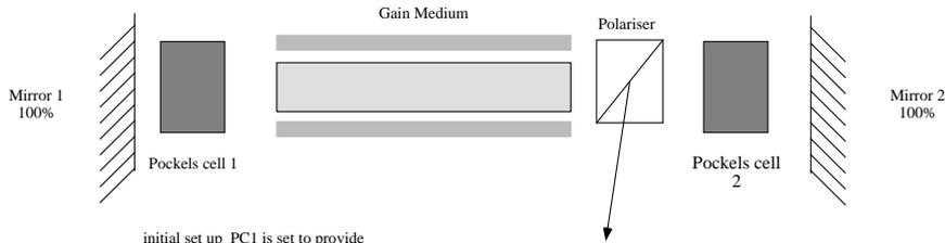
initial set up PC1 is set to provide quarter wave retardation per transit.
