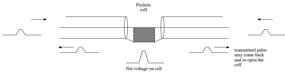
A pulse combining system using two lower voltage pulses. This requires less pulsed power than a single pulse. Although this has a better risetime than a single sided drive it gives rise to reflections at the round trip time of the cabling.
