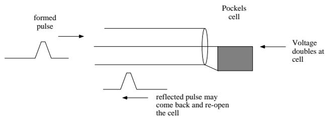
An unterminated system requires half the pulse power but the response is 2 times slower than above. If this is fast enough then one also has to allow for reflections of the pulse from the driver after a round trip time of the cables.
