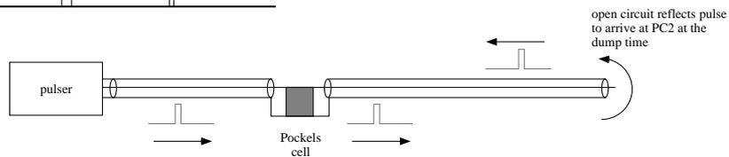
Intra-cavity switching offers significantly increased efficiency over extra-cavity switching but is not so simple to set up or use. It is also less flexible. However, it can obviate the need for further amplification and for fixed configurations can offer a cost effective solution to short pulse generation.
