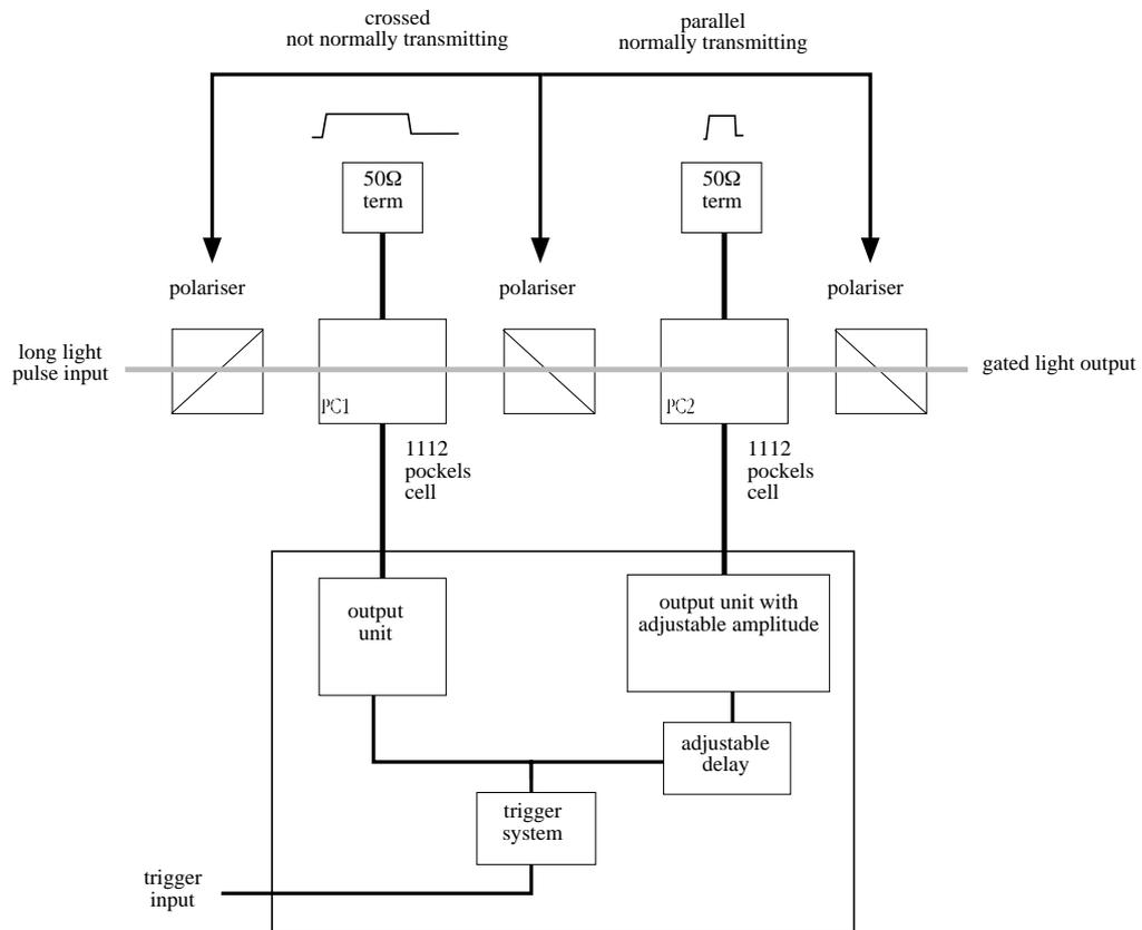
An arrangement for producing an adjustable pulse length from around 120ps to 6ns with both fast rise and fall edges. PC1 delivers the fast rising edge to the light pulse and the long term extinction. PC2 delivers the fast falling edge and reasonable extinction until the pulse drive to PC1 falls and increases the extinction. PC2 cannot maintain good extinction because the extinction is held by the pulse voltage which cannot be stable enough long term.
