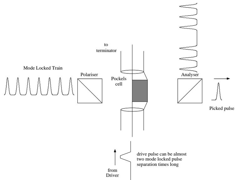
A similar arrangement being used to pulse pick. Driver requirements are somewhat different. The pulse must go from zero to zero in less than two mode locked cycles. If the laser is "Q" switched and mode locked then late time reflections are not important. For CW mode locked lasers there must be no post pulse signals.
