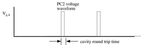
The double pulse on PC2 is conveniently produced by delivering a pulse into a 50Ω cable. The cable is continued after the cell to an open circuit, the reflection from the open circuit delivers the second pulse. This reflected pulse will not be so square as the original but it is always wider than the pulse it has to dump.
