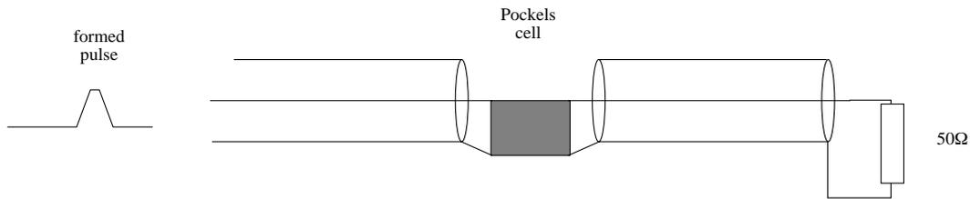
Simplest pulse drive circuit. Can be fast but requires a lot of pulser power. Hard to adjust the pulse length below 500ps but fixed lengths can go to 100ps.
