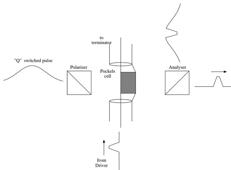
The basic pulse slicing arrangement. This is shown being used to slice a section out of a typical "Q" Switched pulse.
