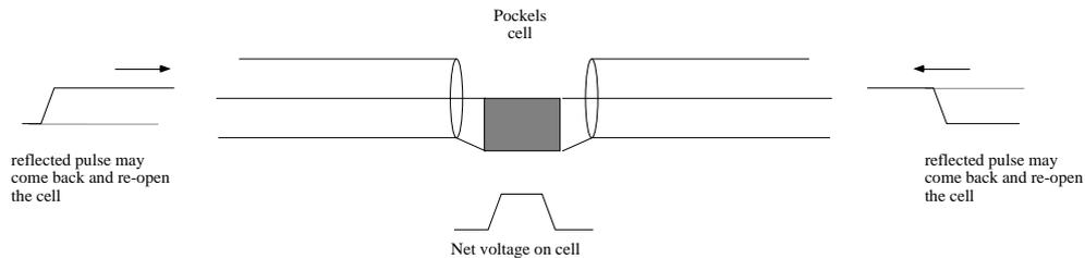
A pulse edge colliding system. The edges can be very fast so that full adjustment down to 100ps is possible. The edges decay in a few ns so this is not good for long pulses. The edges also reflect from the driver after a round trip time of the cables.
