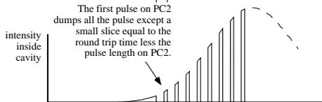
The output pulse length is approximately equal to the round trip time less the length of the pulse first applied to PC 2. Note that as the same pulse is used to dump the cavity as to modulate the pulse within it one can only achieve pulselengths up to half the round trip time with this arrangement. For longer pulses simple cavity dumping may be adequate.
