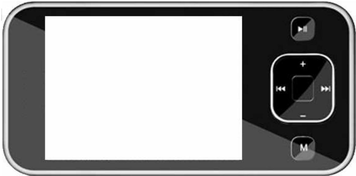
DSO mobile is a pocket size digital storage oscilloscope fulfills basic electronic engineering requirement. It is base on ARM [Cortex™-M3](#) compatible 32 bit platform, equipped with 320\*240 color display, SD card capability, USB connection, and 3.7v chargeable batteries.
