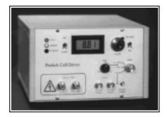
This unit is designed as a Q switch driver, although it may be used for many other applications and has been used for pulse picking. It is based on FET technology and can switch up to 8.5kV to ground in < 5ns via a  $50\Omega$  cable. It will run at up to 200Hz into low capacitance loads. This technology is easily scaled up to higher repetition rates.
