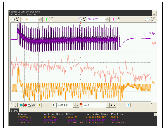
Figure 11. FFT spectrum of PEA signal for AES in PA3.
