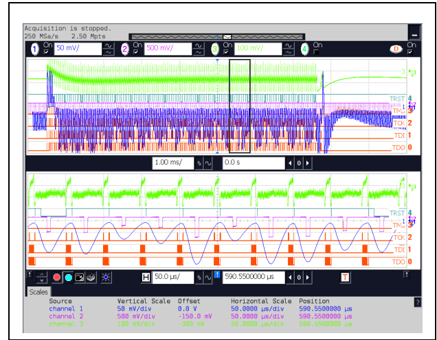
Figure 10. PEA results on PA3 for AES key scanning.
