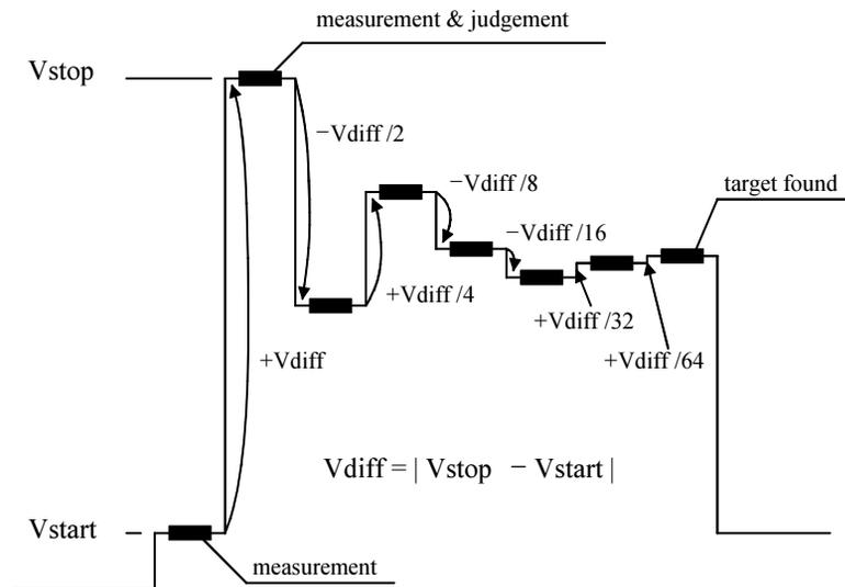
1. The source unit forces  $V_{start}$ , and the monitor unit makes a measurement.
