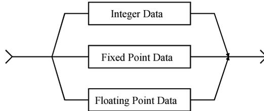
The following 3 figures show the syntax diagrams for integer, fixed point, and floating point data, respectively.
