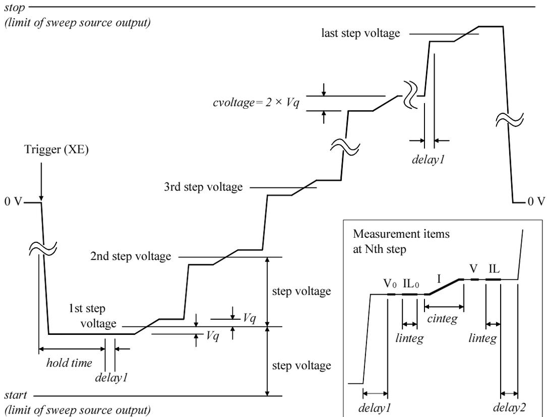
The operation of the quasi-static CV measurements is explained below. This is the case of  $start < stop$ .
