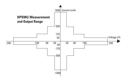
$<sup>^{2}</sup>$  200V (Iout ≤50mA), 100V (50mA<Iout≤125mA), 40V (125mA<Iout≤500mA), 20V (500mA<Iout≤1mA)
